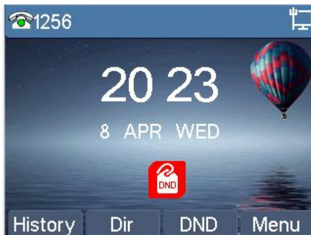
Figure 31 - DND Enabled on All Lines
